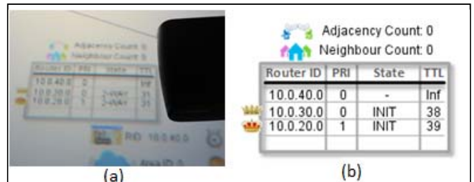
Fig. 7. Topological tables virtually embodied with physical router illustrate internal data held by the device for OSPF execution.
