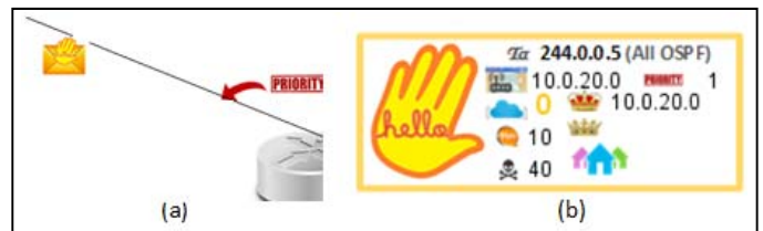
Fig. 8. a) Data exchange animation is visualized by the framework by sequentially displaying the movement of a 'hello' packet. b) Information within the packet is exposed at destination device with image-based indications of the contained values.
